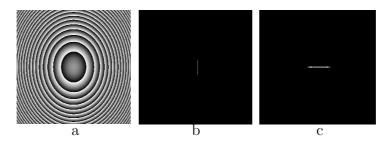
**Figure 3.** Design of a sphero-cylindrical Fresnel lens. (a) Complex amplitude on emitter  $\mathcal{P}$ , corresponding to the phase levels of the lens (represented by grey levels). (b) Focus line at distance 10 mm. (c) Focus line at distance 15 mm. (Numerical simulations.)
