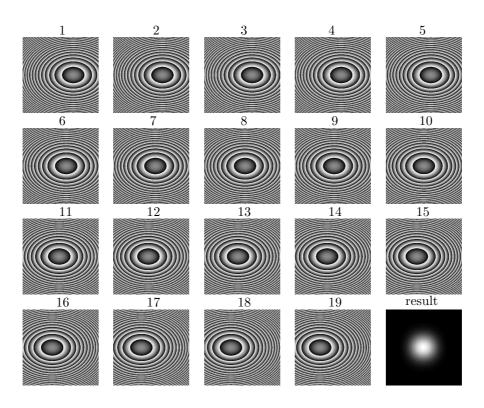
**Figure 9.** The 19 Fresnel lenses to be set in front of the 19 laser diodes. Each lens is appropriately shifted and produces a circular illuminated area, according to Fig. 8. Botton right: the resulting irradiance in the focus plane.
