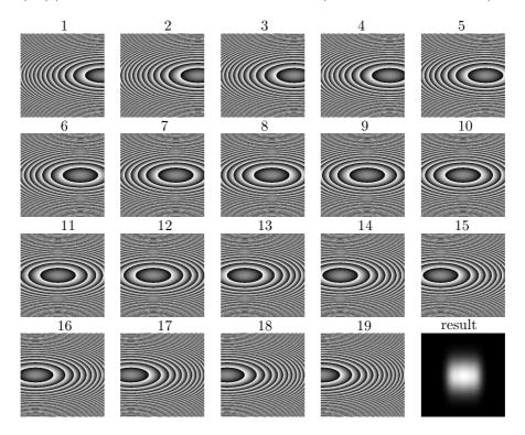
**Figure 7.** The 19 Fresnel lenses to be set in front of the 19 laser diodes. Each lens is appropriately shifted and produces an elliptical illuminated area, according to Fig. 6. Botton right: the resulting irradiance in the focus plane. For display convenience, the lenses are organized in an array: in fact they are aligned along a segment, as the laser diodes.
