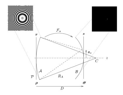
Figure 2. Top left: complex amplitude on emitter  $\mathcal{A}$ , corresponding to the phase of a Fresnel lens (represented by grey levels). Top right: corresponding focus on receiver  $\mathcal{B}$ . The lens is not centred, so that the focus on  $\mathcal{B}$  is shifted by  $s_0$ . Parameters in the figure are spatial ones; scaled parameters are needed for actual simulations, according to Eq. (9).
