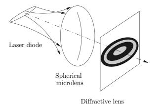
**Figure 5.** Optical set up for each one of the 19 laser diodes (see Fig. 1). The laser diode emits a Gaussian beam with elliptical waist. A spherical refractive microlens is set in front of the laser diode. The astigmatic Gaussian beam incident on the diffractive lens has two one-dimensional waists.
