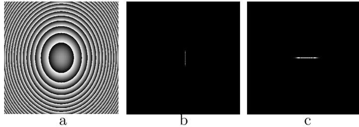
**Figure 3.** Design of a sphero-cylindrical Fresnel lens. (a) Complex amplitude on emitter  $\mathcal{P}$ , corresponding to the phase levels of the lens (represented by grey levels). (b) Focus line at distance 10 mm. (c) Focus line at distance 15 mm. (Numerical simulations.)
