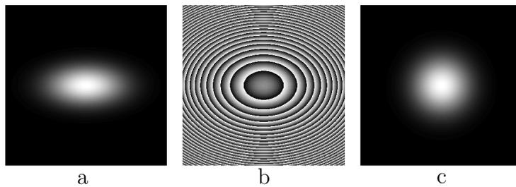
**Figure 8.** Focusing an astigmatic Gaussian beam on a circular area. (a) Gaussian beam irradiance in the lens plane. (b) Phase levels of the sphero-cylindrical Fresnel lens (represented by grey levels). (c) Irradiance at 30 mm from the lens. (Numerical simulations.)
