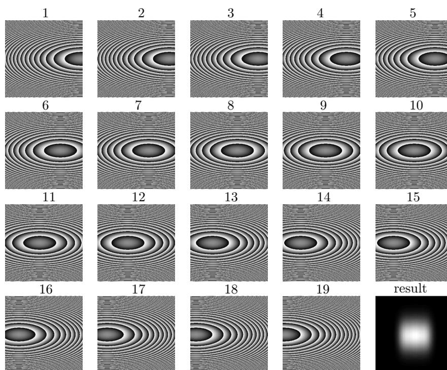
**Figure 7.** The 19 Fresnel lenses to be set in front of the 19 laser diodes. Each lens is appropriately shifted and produces an elliptical illuminated area, according to Fig. 6. Bottom right: the resulting irradiance in the focus plane. For display convenience, the lenses are organized in an array: in fact they are aligned along a segment, as the laser diodes.
