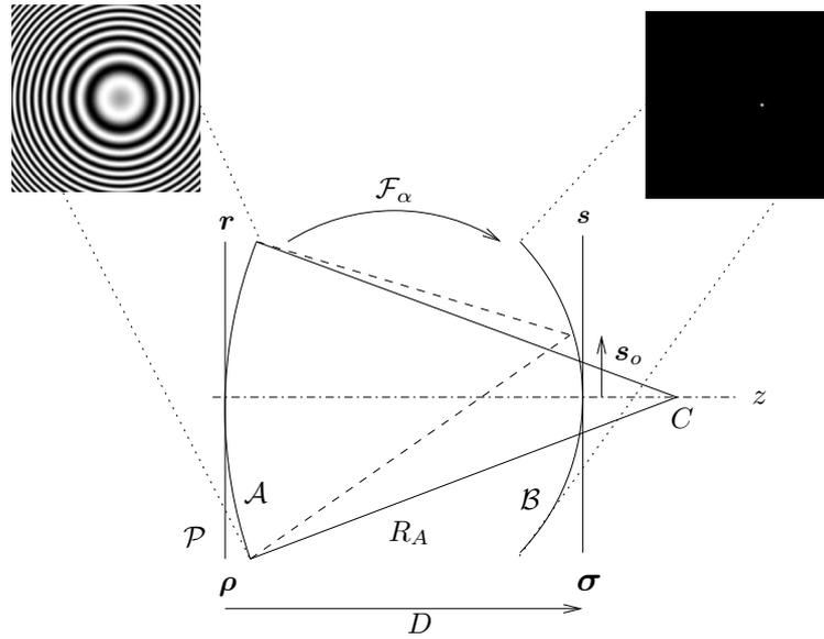
**Figure 2.** Top left: complex amplitude on emitter  $\mathcal{A}$ , corresponding to the phase of a Fresnel lens (represented by grey levels). Top right: corresponding focus on receiver  $\mathcal{B}$ . The lens is not centred, so that the focus on  $\mathcal{B}$  is shifted by  $\mathbf{s}_0$ . Parameters in the figure are spatial ones; scaled parameters are needed for actual simulations, according to Eq. (9).
