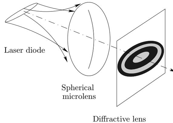
**Figure 5.** Optical set up for each one of the 19 laser diodes (see Fig. 1). The laser diode emits a Gaussian beam with elliptical waist. A spherical refractive microlens is set in front of the laser diode. The astigmatic Gaussian beam incident on the diffractive lens has two one-dimensional waists.
