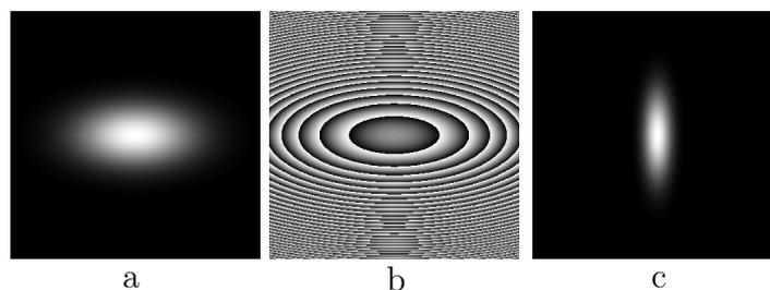
**Figure 6.** Focusing an astigmatic Gaussian beam on an elliptial area. (a) Gaussian beam irradiance in the lens plane. (b) Phase levels of the sphero-cylindrical Fresnel lens (represented by grey levels). (c) Irradiance at 30 mm from the lens. (Numerical simulations.)
