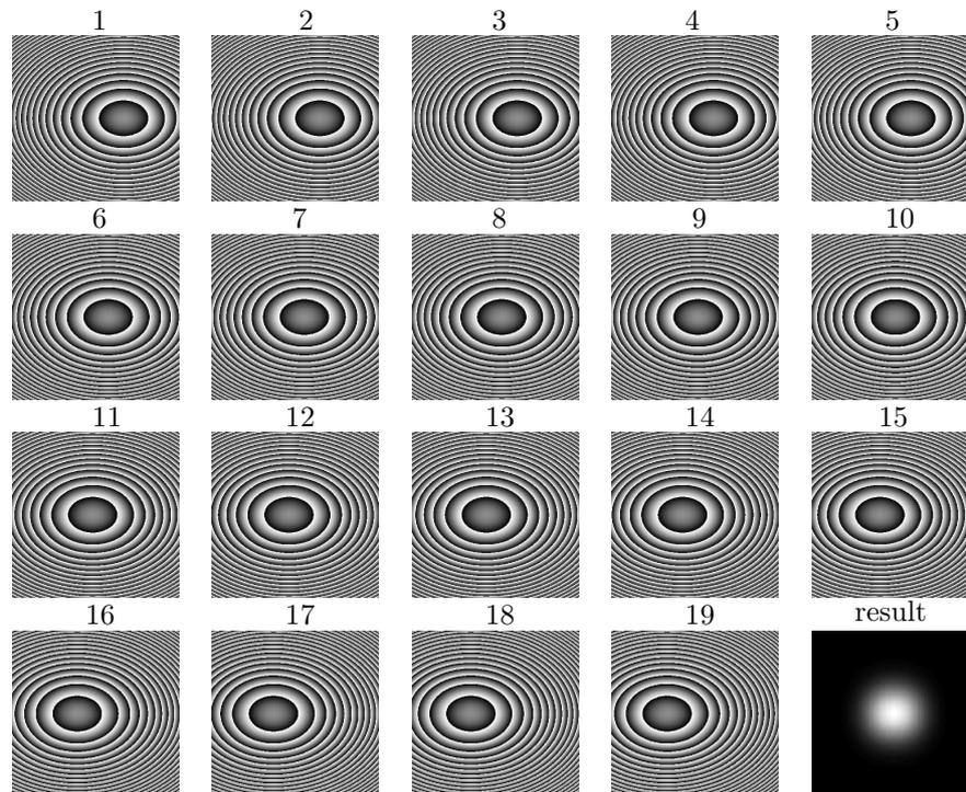
**Figure 9.** The 19 Fresnel lenses to be set in front of the 19 laser diodes. Each lens is appropriately shifted and produces a circular illuminated area, according to Fig. 8. Bottom right: the resulting irradiance in the focus plane.
