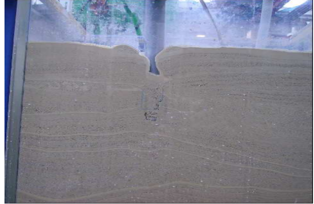
Figure 14: stratification after underwater compaction
