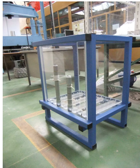
Figure 2: The tank used with the two boreholes and the pumping system
