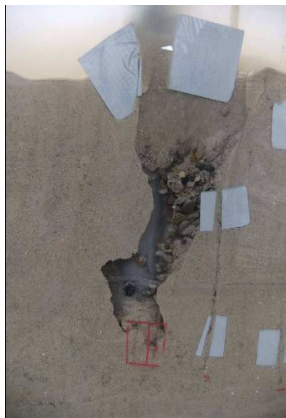
Figure 15 : soil boiling close to injection pipe
