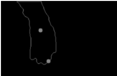
Figure 6: when fingers are closed separation of fingers in the depth image is not possible
