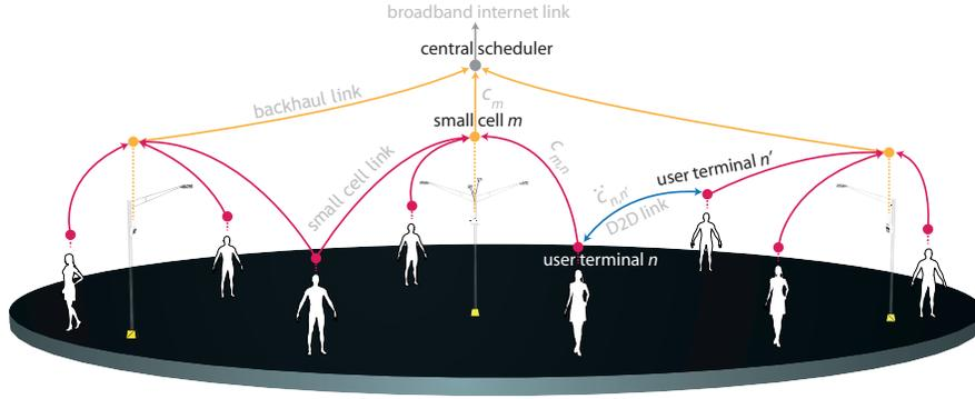
Figure 1: An illustration of the studied network deployment. A central scheduler communicates with  $M$  SBSs via backhaul links. In addition to their cellular connections, D2D communication among socially-connected users is depicted.
