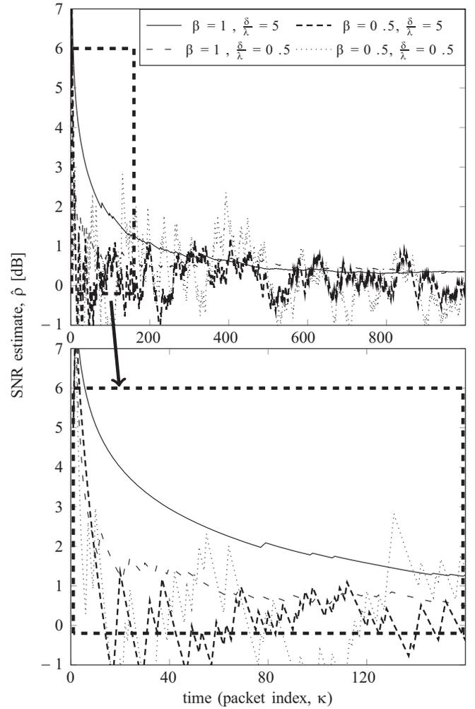
Fig. 2. Illustration of the trajectory of the SNR estimator.  $\beta \in \{0.5, 1\}$  and  $\frac{\lambda}{\lambda} \in \{0.5, 5\}$ .
