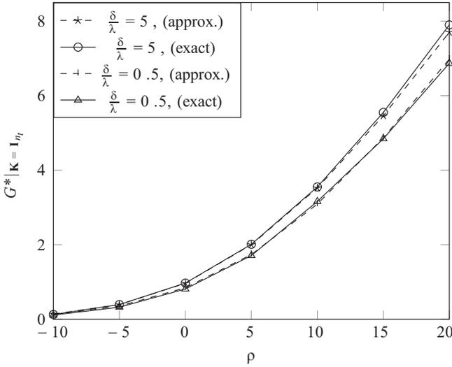
Fig. 1. Optimal goodput of a 2x2 MIMO system from Monte-Carlo simulation (exact) and Gaussian approximation (app.), with high ( $\frac{d}{\lambda} = 0.5$ ) and low ( $\frac{d}{\lambda} = 5$ ) spatial correlation.
