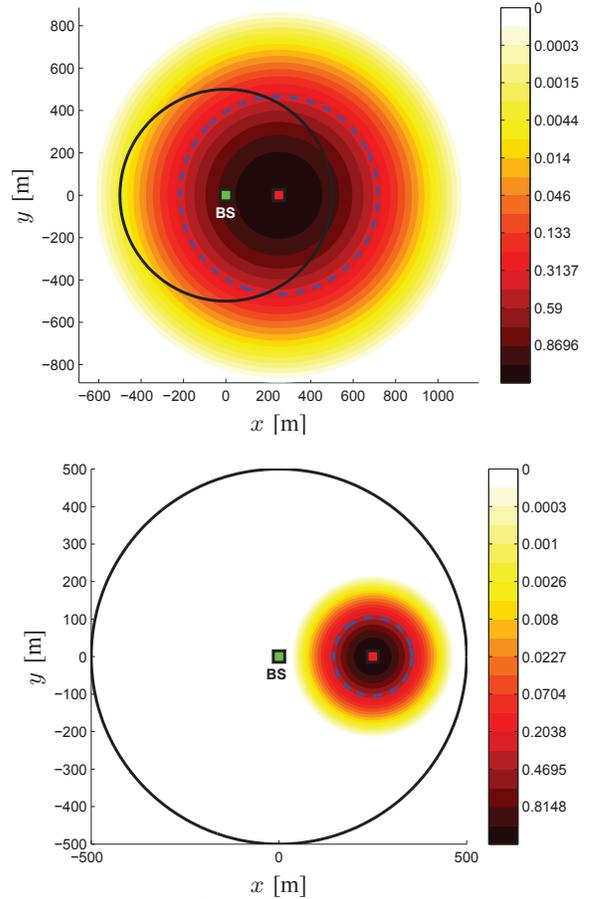
Fig. 3. Probability of D2D mode optimality for (P1) (top) and (P2) (bottom) with  $N = 8$ ,  $p_{\text{UE}}^* = 15$  dBm,  $R^* = 4$ , and  $d_h = 250$  m. The color shows the probability for D2D mode optimality when the receiving UE is at different locations. The black circle is the cell boundary and the dashed blue one is the boundary of D2D optimality area based on only path-loss information.
