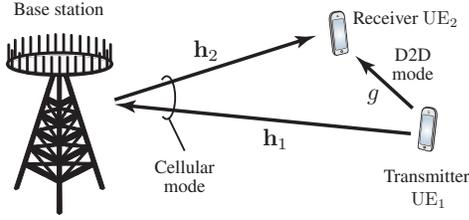
Fig. 1. Illustration of the system model where UE<sub>1</sub> communicates with UE<sub>2</sub>, either via the BS (cellular mode) or by direct transmission (D2D mode).
