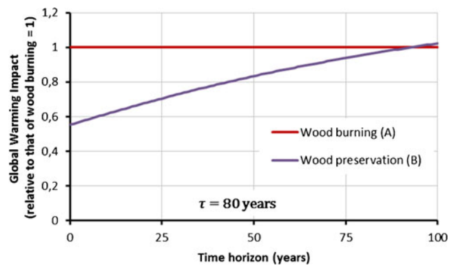
Fig. 5 Global warming potential of option B (gas burning, wood being preserved) relative to that of option A (wood burning) taken as the reference. See example of Fig. 2. The time constant of wood degradation is supposed to be 80 years (half-life of 55 years)
