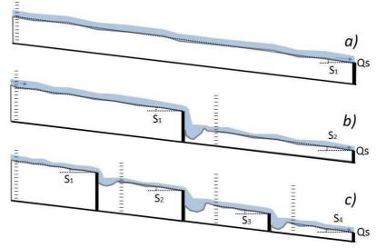
Figure 1. Sketches of the different setup: a) Ref Test; b) 1GCS Test; c) 3 GCS Test.
