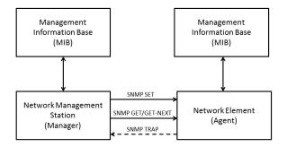
Fig. 2: SNMP architecture and operations.
