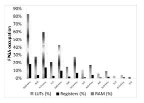
Fig. 6: FPGA occupation for synthetic traffic implementation
