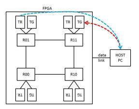
Fig. 1: hardware implementation of TGs and TRs.
