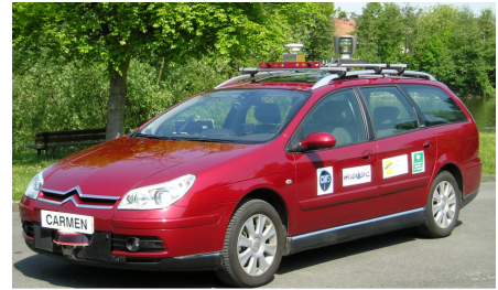
Figure 8: Experimental platform with the Velodyne sensor
