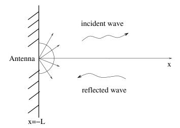
Figure 1: X-mode in slab geometry: the domain. In a real physical device an antenna is on the wall on the left and sends an incident electromagnetic wave through a medium which is assumed to be infinite for simplicity. The incident wave generates a reflected wave which can be used to identify the properties of the plasma. The medium is filled with a plasma with dielectric tensor given by (3).
