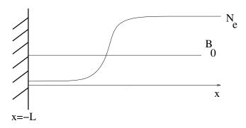
Figure 2: The physical parameters for the X-mode equations in slab geometry. The electronic density  $x \mapsto N_e(x)$  is low at the boundary, and increases towards a plateau. The background magnetic field  $B_0$  is here taken as constant for simplicity.
