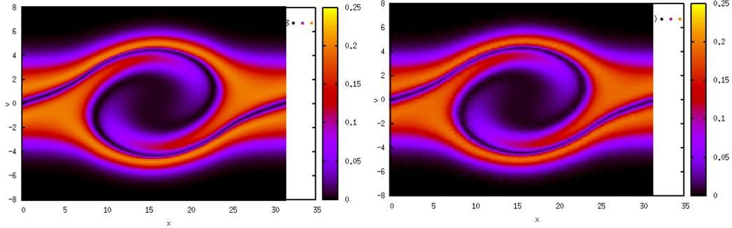
Figure 2: The distribution function of the two-stream test case at time  $t = 25$ . The first coordinate is the space coordinate  $x_1$ . The second coordinate is the velocity  $v_1$ . Left: reduced Vlasov-Poisson method. Right: the PIC method.
