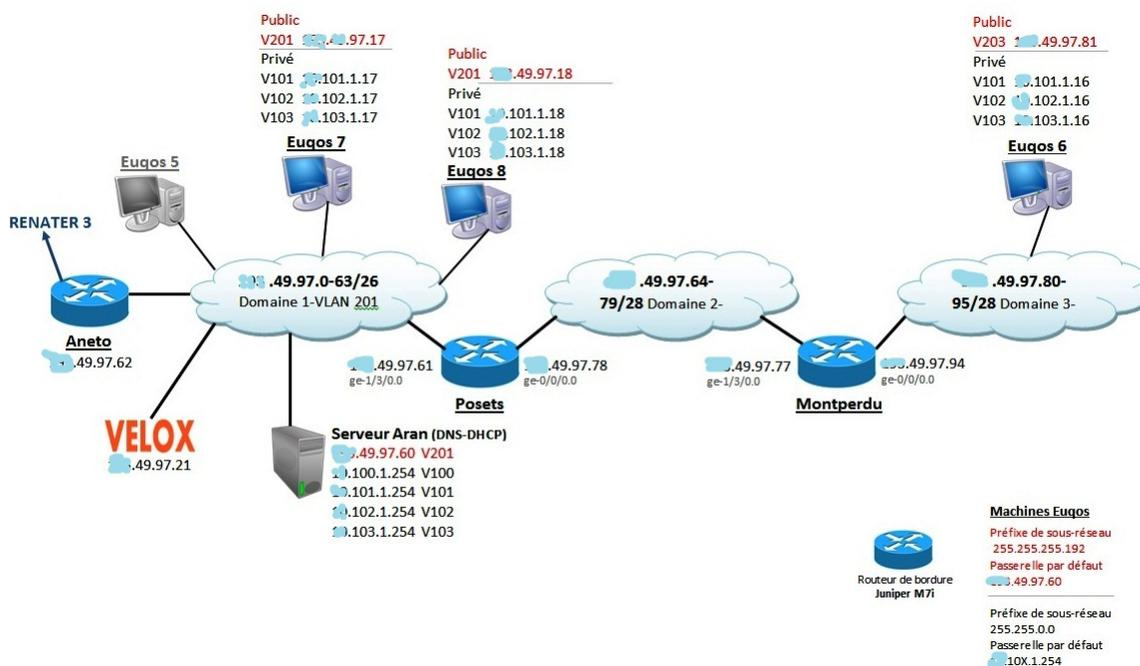
FIGURE 8: Laasnetexp testbed
