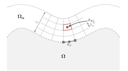
Fig. 4.2: Definition of the mesh  $\mathfrak{M}_{\alpha}$
