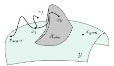
Fig. 2. Illustration of the tree exploration in the state space  $\mathcal{X}_{adm}$  while sampling states on the submanifold of quasi-static contact-free states  $\mathcal{Y}$ . We can see that the resulting state of an extension step can lie on this submanifold as  $x_i$ , be in contact as  $x_k$  or be any state in  $\mathcal{X}_{adm}$  as  $x_j$ .
