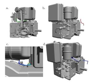
Fig. 7. Start (in green at clipped view a) and goal (in red at view b) states for the disassembly scenario "engine". The solution path makes use of contacts (views c and d).
