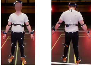
Fig. 1. Front and back pictures of the equipped subject, including 12 on-body HikoB nodes and tens of Vicon markers.
