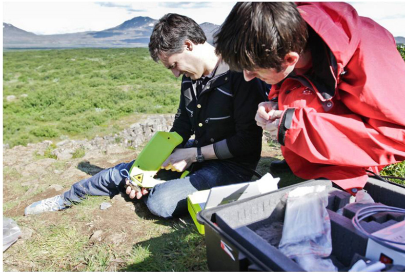
Fig. 1. Portable LIBS system and its two main parts, connected together by an umbilical. Photo from J.-F. Buoncristiani.
