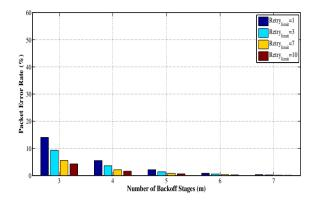
Fig. 13. Packet error rate for #band=4 vs. number of backoff stages for various retransmission limits.
