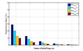
Fig. 11. Packet error rate for single band vs. number of backoff stages for various retransmission limits.
