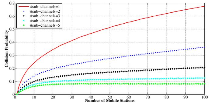
Fig. 4. Collision probability vs. number of mobile stations for various RTS bands number.
