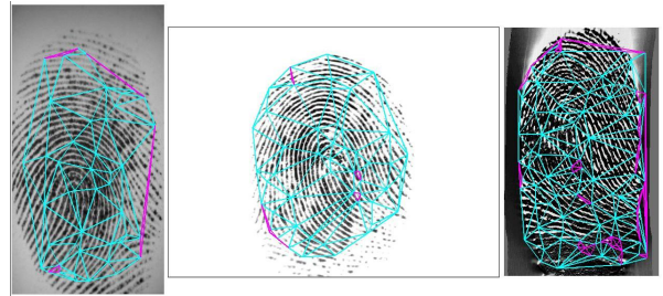
Figure 3: Example of minutiae Delaunay triangulations of 3 different FVC images. NFIQ values are 2, 2 and 1, respectively.
