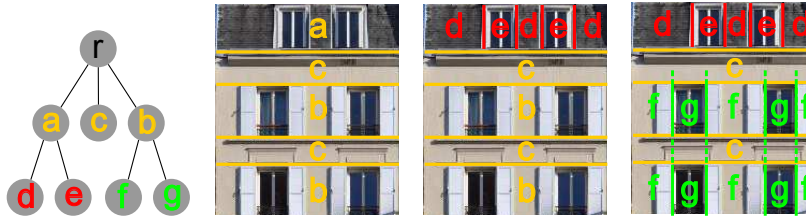
Fig. 1. A shape prior consists of a hierarchy of classes (image 1) and a table of pairwise potentials for each nonterminal node (not shown here). Each image (2-4) shows substitution of all rectangles of a particular class with rectangles of child classes.
