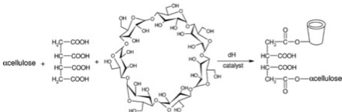
Fig. 1. Attachment of BCD to cotton with BTCA. 5 Source reproduced with permission from Elsevier.
