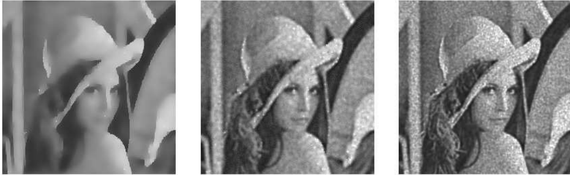
Figure 2: The restoration results by three models when m = 50 . Left: PM equation (3.2); Middle: YK equation (1.2); Right: our model (3.1).
