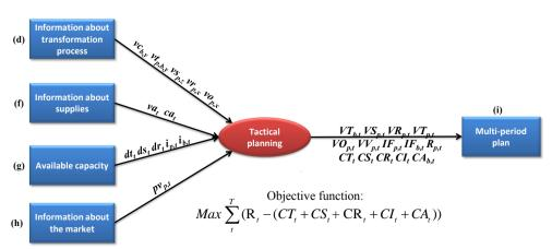
Figure 5: Outputs and inputs of the tactical planning model
