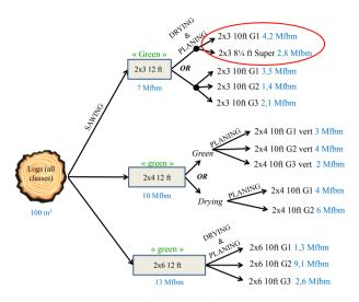
Figure 7: New mix of products for the product 2x3 12ft enabling producing the new product (2x3 81/4ft Super)
