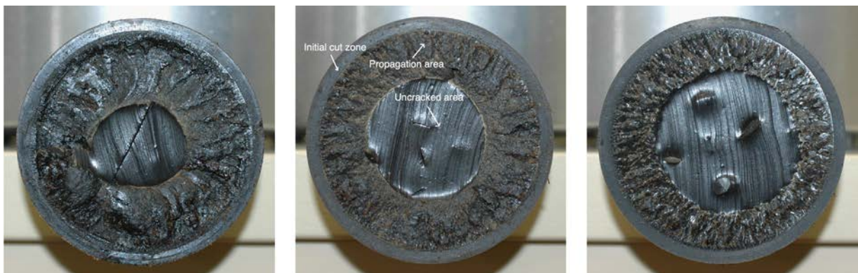
Fig. 6. Fracture surfaces for a given axial displacement. Left: 0.3 mm (sample FU3), middle: 0.5 mm (sample FU1), right: 1 mm (sample FU4).
