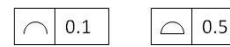
Figure 1: Form specifications of a profile of a line and of a surface
