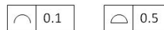
Figure 1: Form specifications of a profile of a line and of a surface
