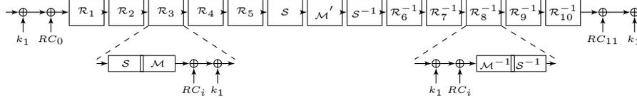
**Fig. 2.** Structure of the core of PRINCe
