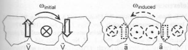
Fig. 4. The Lenz law in physical mesomechanics. Solid arrows represent velocity caused by the initial rotation due to an external torque and dashed arrows represent induced acceleration
