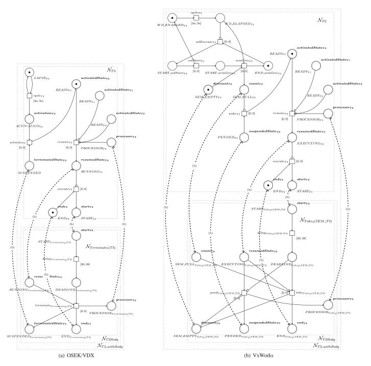
Fig. 6: RI\_TPN of periodic task implemented on two different RTOS
