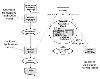
Fig. 3: Multi-platform deployment process within SExPIsTools
