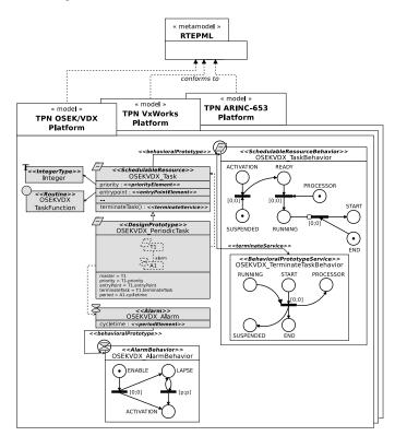
Fig. 2: Behavioral representation of OSEK/VDX platform
