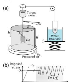
FIG. 1: (a) Experimental set-up. (b) Imposed stress during an experiment: stress ramp to reach mean stress,  $\sigma_0$ , constant stress during  $t_w$  and stress modulation characterized by a frequency  $f_{\sigma}$  and an amplitude  $\delta$ .
