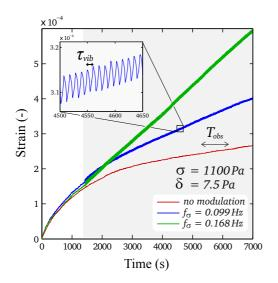
FIG. 2: Strain as a function of time for three experiments performed at  $\sigma_0 = 1100$  Pa, and  $\delta = 7.5$  Pa, and for various oscillations frequencies. The oscillations start at t = 1500s (grey area).
