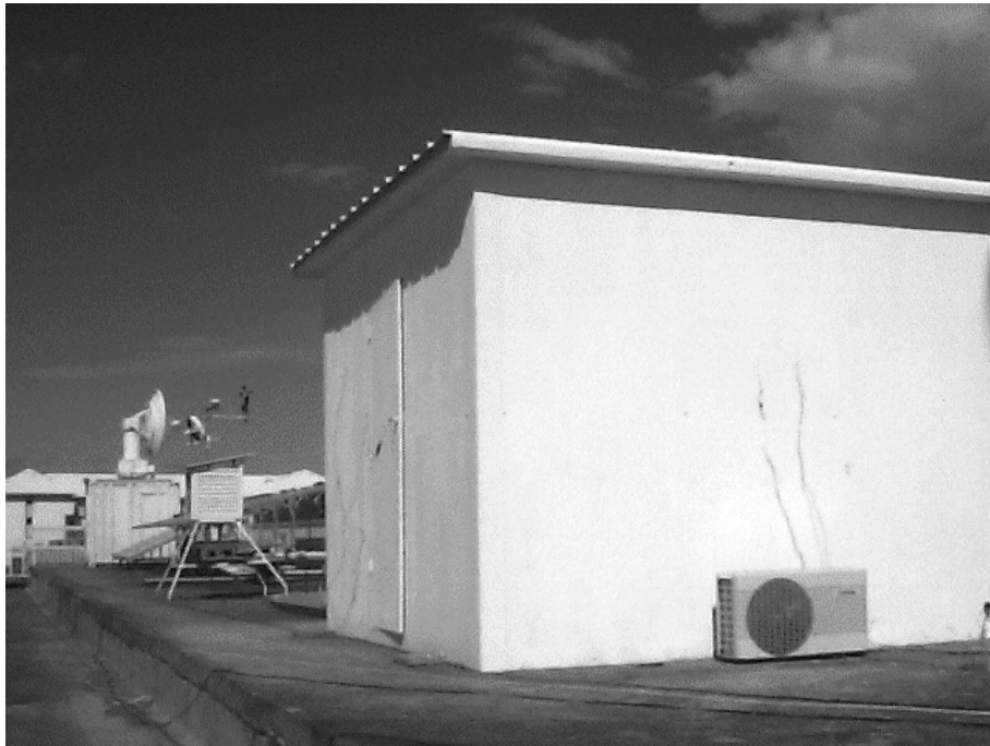
Figure 4 : Picture of the test cell and in the back, the weather station that provides solicitations to the model
