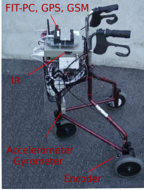
Fig. 1. The instrumented walking aid. Fig. 2. Simple kinematic model of the walker.
