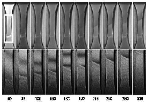
Fig. 1 Lüders' front (upper) and WB (lower) observed simultaneously at the crosshead speed of  $2.5 \mu\text{m/s}$ . Numbers represent the elapsed time in s from a reference time set before the yield point. The window inserted in the leftmost image of the upper row indicates the view of the lower images approximately.
