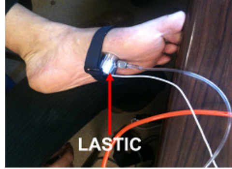
Figure 3. Acquisition of the elastic modulus of the skin below the foot arch using LASTIC.
