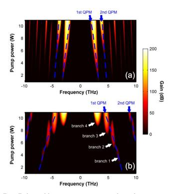
Fig. 1. Evolution of the output gain spectrum according to the input power for an average dispersion of 0.7 ps<sup>2</sup>/km (a) and 0.13 ps<sup>2</sup>/km (b). The corresponding pumping wavelengths are 1536 and 1554 nm. Results are obtained from the linear stability analysis based on the Floquet theory. The predictions from Eq. (3) are plotted with blue line.
