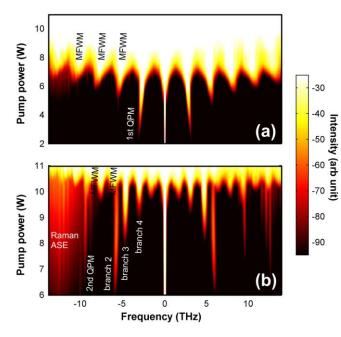
Fig. 5. Evolution of the output spectrum according to the power for a pump wavelength of (a) 1536 nm and (b) 1554 nm. Results obtained from the numerical integration of the extended NLSE. Results are averaged over 36 simulations.
