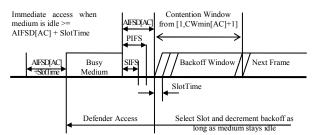
Fig. 2. IEEE 802.11e EDCF channel access
