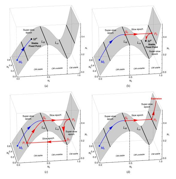
**Figure 6:** Outline schematic showing the possible steady-state regimes of the full slow-flow system (49): (a) a stable fixed point  $M^e = \begin{bmatrix} n_1^e & n_2^e & n_3^e & \delta_{21}^e & \delta_{31}^e \end{bmatrix}^t$  with  $n_2^e < N_{2,M}$  is reached, (b) a stable fixed point  $M^e = \begin{bmatrix} n_1^e & n_2^e & n_3^e & \delta_{21}^e & \delta_{31}^e \end{bmatrix}^t$  with  $n_2^e > N_{2,M}$  is reached, (c) relaxation oscillations and (d) explosion.
