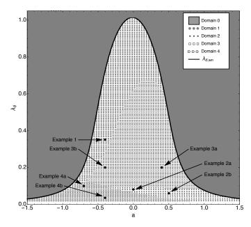
**Figure 10:** Prediction, in the plane  $(\lambda_{\delta}, a)$ , of the domains of existence of the four steady-regimes: *Complete suppression* (the gray area outside the curve  $\lambda_{\delta, \operatorname{wn}}(a)$ ), *Partial suppression through Periodic Response* ( $\bullet$ ), *Partial suppression through Strongly Modulated Response* ( $\Box$ ) and *no suppression* ( $\Box$ ). Parameters used: see Eq. (85).
