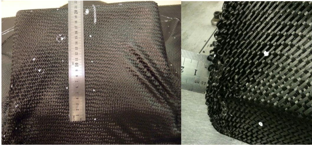
(a) Buckles and wrinkles on the side face
