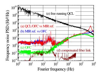
**Figure 3. Frequency noise Power Spectral Density (PSD)** of (a) the beat note between the QCL phase-locked onto the NIR reference (QCL/OFC) and the MIR reference (red), (b) the beat note between the MIR reference and the OFC (blue), (c) the OFC (green), (d) the noise compensated 43-km optical fibre link (brown) and (e) the free running QCL (black). All these PSDs are relative to a carrier frequency of 29.1 THz (10.3-µm wavelength).
