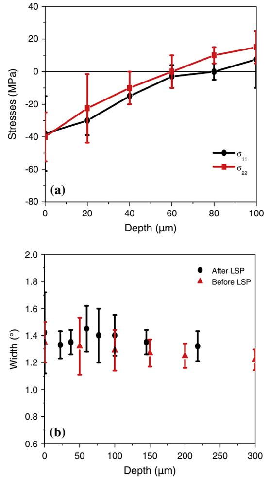
**Fig. 6.** (a) Initial residual stresses of AA2050-T8,  $\sigma_{11}$  (rolling direction) and  $\sigma_{22}$  (transverse direction), (b) influence of LSP on the integral widths of X-ray peaks (5  $\text{GW}/\text{cm}^2$  – 50% overlap).
