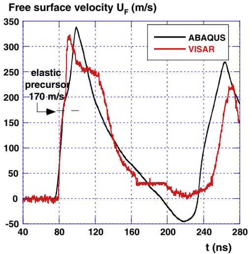
Fig. 5. Determination of the elastic precursor (inflexion at 170 m/s) and shock yield stress using back free velocity  $U_F$  measurements on a 430 μm-thick 2050-T8 foil ( $I = 5.5$  GW/cm<sup>2</sup>, surface pressure = 3.8 GPa)-comparison with Abaqus simulation.
