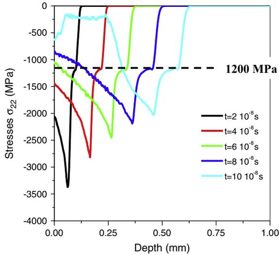
**Fig. 10.** Stress wave propagation for a  $P = 3$  GPa incident pressure corresponding to  $I = 3.5$  GW/cm<sup>2</sup>.
