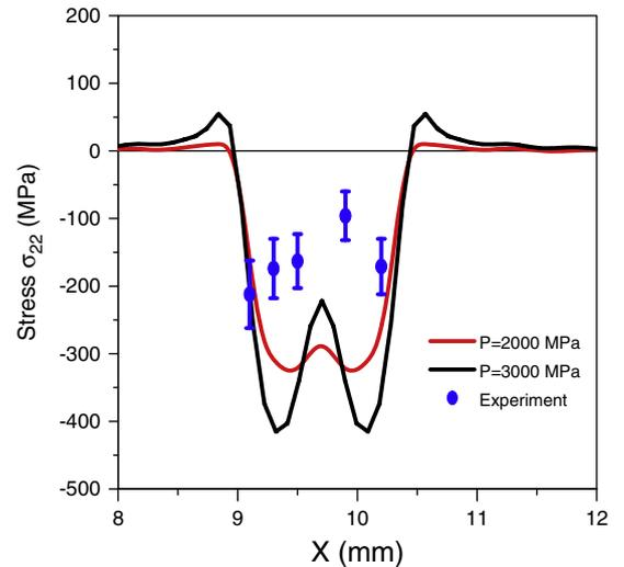
**Fig. 12.** FEM simulation of residual stresses induced by a 1.5 mm impact for 2 and 3 GPa. Comparison with  $\mu$ XRD measurements carried out on a single 3.5 GW/cm<sup>2</sup> impact.
