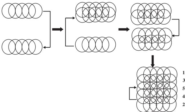
**Fig. 19.** Surface treatment with a non-continuous LSP path.
