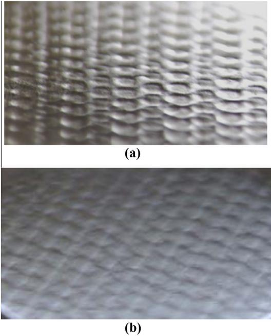
Fig. 3. Surface topography after – (a) a 33% overlap LSP, (b) a 50% overlap LSP (1.5 mm spot diameters, 5 GW/cm<sup>2</sup> power density).
