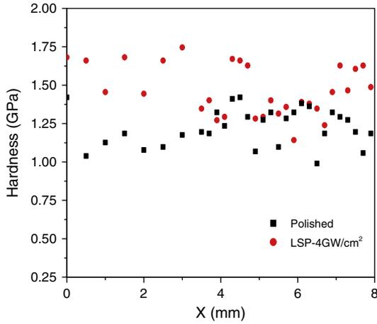
Fig. 7. Vickers hardness distribution after LSP treatment (5 GW/cm<sup>2</sup> – 50% overlap).
