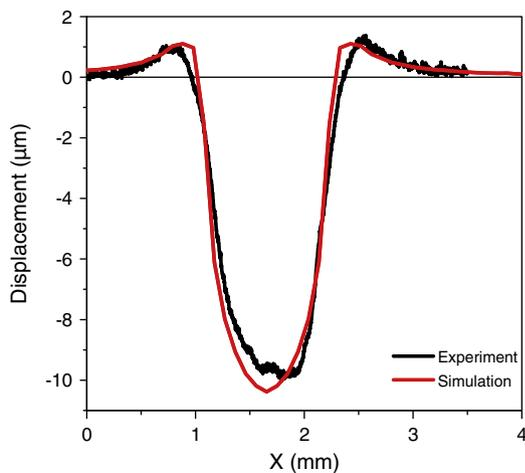
**Fig. 11.** Comparison between experimental and simulated single laser impact: 1.5 mm – 8 GW/cm<sup>2</sup> impact (5 GPa) simulation with a spherical  $P = f(x, y)$  distribution.
