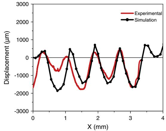
**Fig. 15.** Experimental versus simulated surface deformation  $u_{33}$  induced by 25 laser impacts ( $1.5 \text{ mm} - 3.5 \text{ GW/cm}^2 - 50\%$  overlap) – simulation with a spherical  $P = f(x,y)$  distribution and  $P = 3 \text{ GPa}$  maximum pressure.
