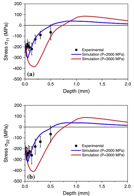
Fig. 17. Influence of impact pressure on in-depth residual stress profile ( $d = 1.5$  mm, 50% overlap) (a)  $\sigma_{11}$ , (b)  $\sigma_{22}$  (simulation results are averaged values using 12 in-depth profiles considered inside a 1.5 mm diameter circular area similar to XRD spot).
