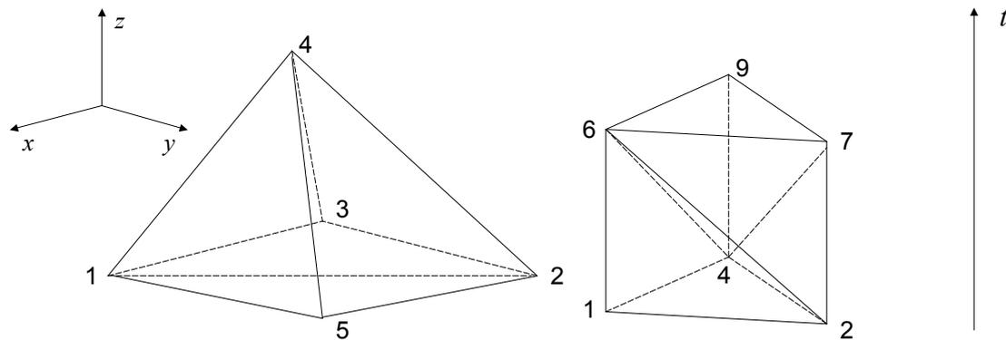
**Figure 4.** 3D initial mesh (scheme at the left); part of the 4D mesh generated by the triangle (1; 2; 4) common to the two finite elements of the 3D initial mesh (scheme at the right).
