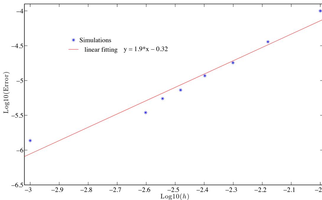
**Figure 8.** Maximum error over the space, at the last time step, between the analytic solution and the numerical solution for each mesh size  $h$ , in the logarithmic scale.
