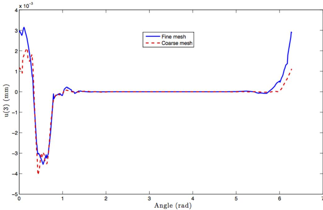
**Figure 11.** Comparison of vertical displacements for points situated on the circle of control, expressed in mm, at time  $t = 2.10^{-5}$  s. Each check point is defined by its angular coordinate, expressed in radians.
