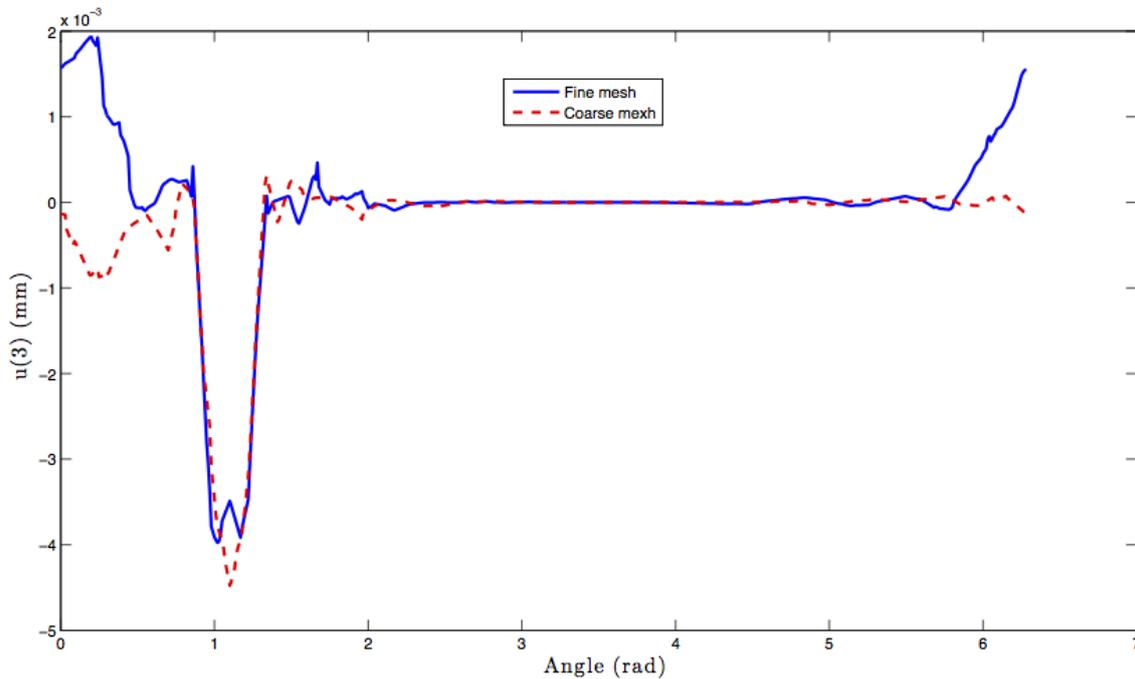
**Figure 12.** Comparison of vertical displacements for points situated on the circle of control, expressed in mm, at time  $t = 4.10^{-5}$  s. Each check point is defined by its angular coordinate, expressed in radians.
