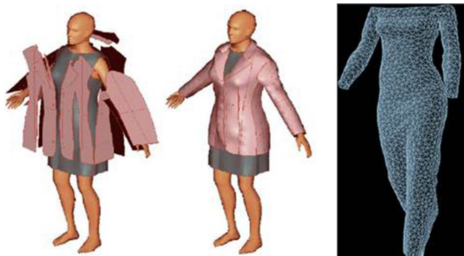
Fig. 2. A 2D-to-3D transformation and simulation model used in the textile industry, adapted from [15] and [16].
