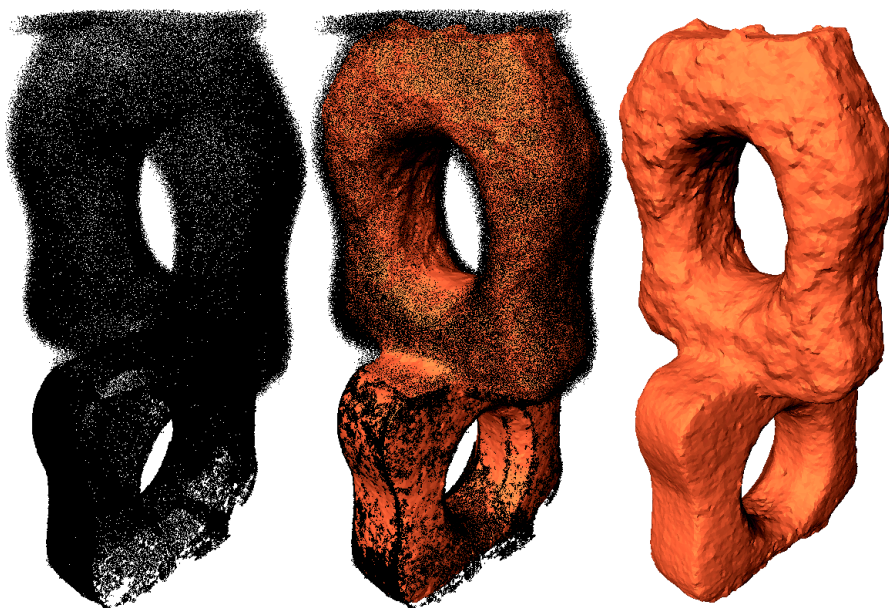
Figure 2.7: Two levels of noise . Left: raw point set with additional noise on the top half part. Middle: point set & reconstruction. Right: reconstruction only (running time: 242s).
