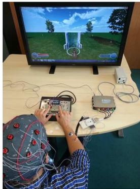
Figure 2 – Notre prototype d'interface BCI hybride
