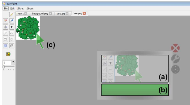
Figure 3. WallPad in a drawing application. The widget comprises a rectangular touch sensitive area (a) with a button below (b). Finger drags in the touch sensitive control the relative position of the pointer (c). The region around the pointer is displayed in the touch sensitive area. Each WallPad button and pointer have a unique color to help disambiguating them.
