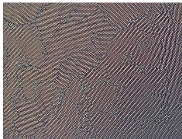
Figure 3: Microscope image (x100) of HCP silica microspheres ( \varnothing 1.1 \mu\text{m} ) displaying grains separated by fracture lines.
