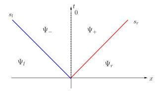
Figure 1: HLLC solver wave pattern
