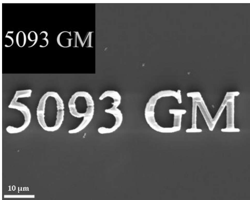
Figure 7. SEM image of a \mu -structure fabricated upon excitation at 800 nm of the diacrylate resin with O g as 2PA sensitizer. Inset: 2D model master.
